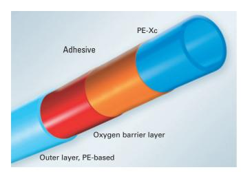
PEX-4-Pipes are designed for heating applications and drinking water installations. They feature an additional oxygen barrier layer as well as an outer protective PE layer. Thus, the oxygen barrier is effectively protected against mechanical damage, ensuring extremely safe installation and operation. PEX-4-Pipe is created in a special coextrusion procedure in which the basic pipe is coated three times in a single production step with three additional layers featuring tight tolerances.
