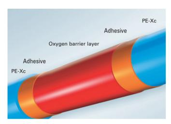
Using a newly developed extrusion procedure, Hewing can process five layers into a homogenous pipe in a single production step. Following subsequent final cross-linking, the pipe is finished: the Penta-Pipe, featuring a centrally positioned oxygen barrier layer. It is equipped with a particularly robust PE-Xc outer pipe, securely connected to the oxygen barrier via a further adhesive layer. Thus, Penta-Pipe is protected from damage on construction sites as well as in operation.
